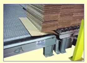
Bottom Sheet is joined to bottom of stacks as it advances forward. **C&M's Sheet Insertion** System provides operator with smooth roller less surface to work.
